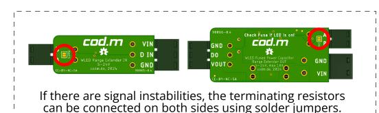
Add WLED Fused Capacitor Board (90062) to additional power connections.
